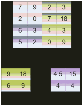
Fig. 6: Max-pooling and average-pooling operations of down-sampling/pooling layer
